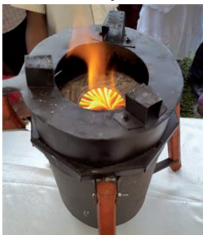
Figure 4. A top lit updraft gasifier stove using solid fuel in an efficient manner, developed by Awamu.
