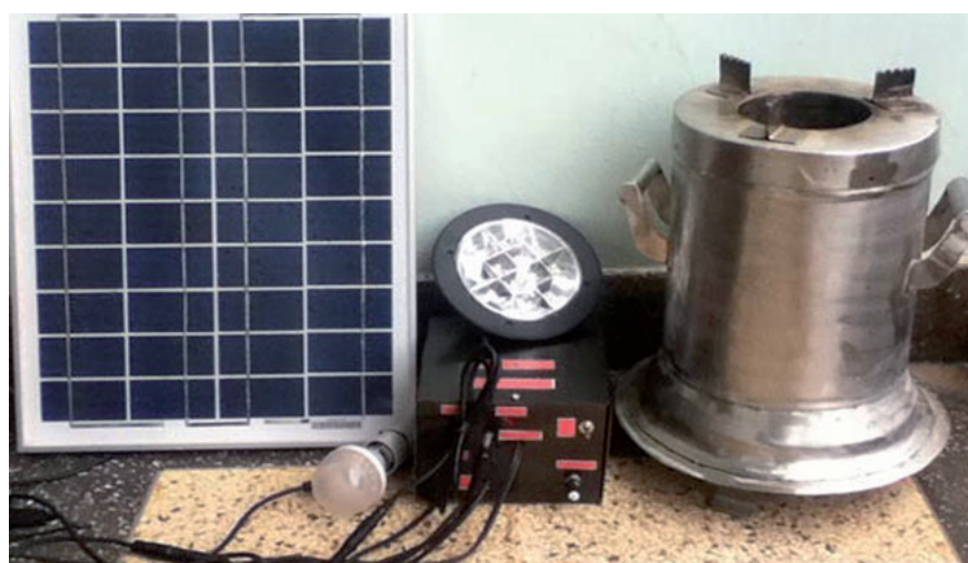
Figure 7: A TERI cookstove with an integrated solar panel
